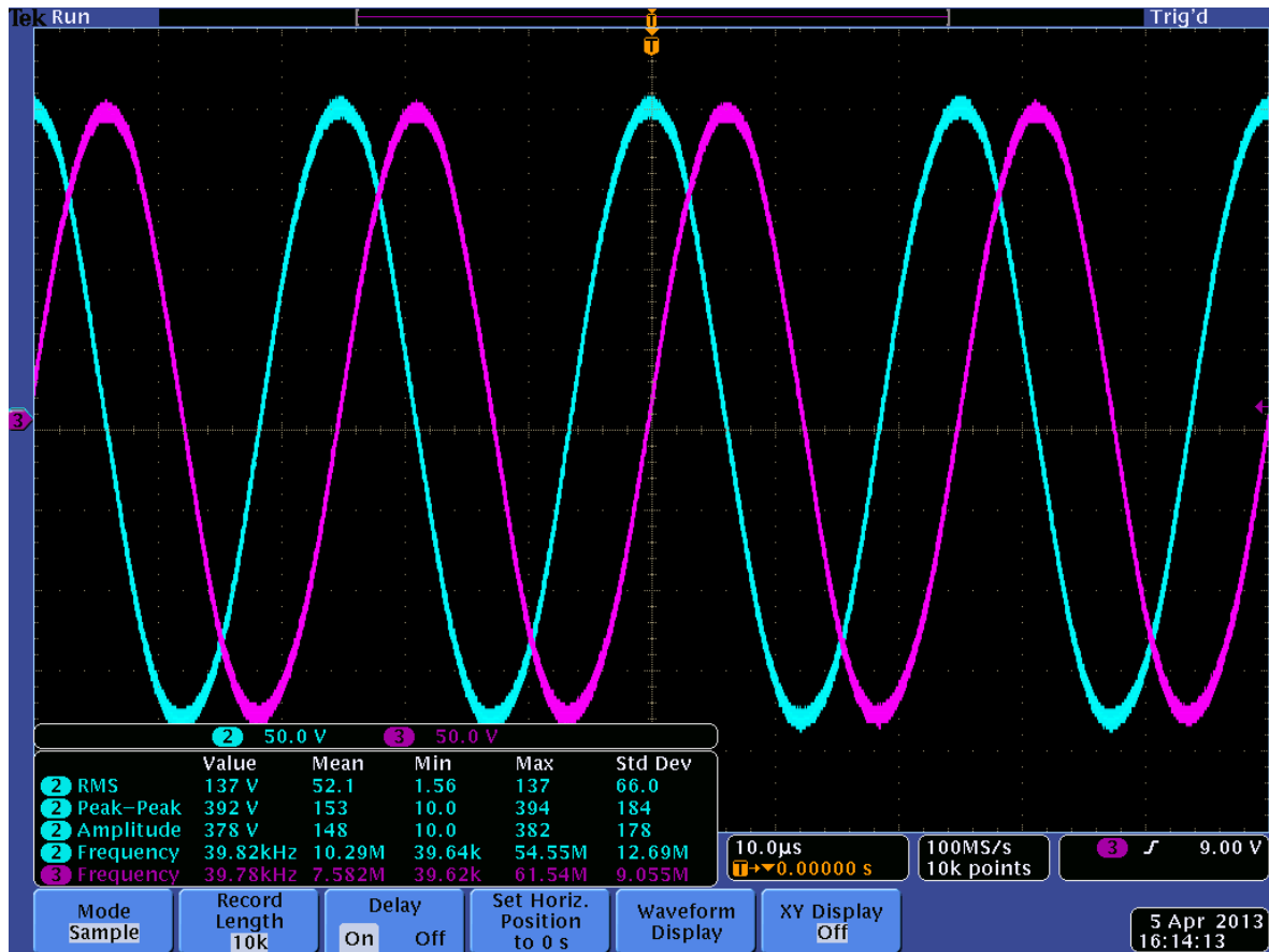
Figure 3. 19: The two waveforms for ultrasonic Shinsei motor
